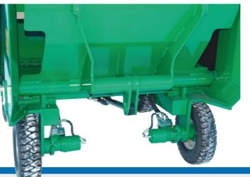
The four-wheel drive is controlled via joysticks. The system is equipped with a differential control valve which acts as a lock for the differential gear. This makes straight driving extremely easy.
