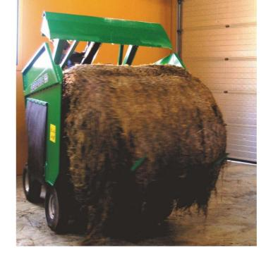
The bale sits on the lift for the duration of the entire work stage. The lift height also determines the length of the chop. Due to the special structure of the lift, the bale can also be removed if necessary. Additional forks are also available for the lift to facilitate handling of loose feed.
