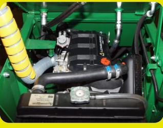
The engine compartment can be opened without any tools for daily checks. The engine with its accessories are situated in a sheltered, but well-ventilated engine compartment which prevents e.g. feed from getting in. Also animals are safe from any hot parts. The block heater is standard equipment.
