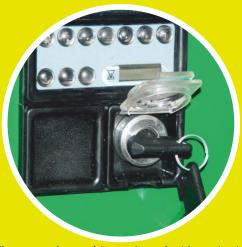
The control panel is equipped with an ignition key, hour meter and engine monitoring system. The main switch is standard equipment.
