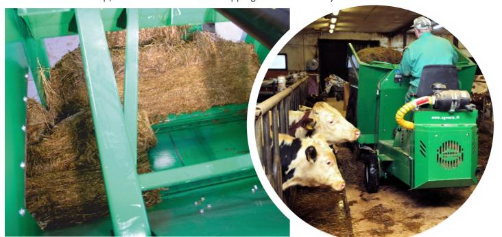
The side conveyor outlets are big enough to push out even the biggest clumps without any problems. The conveyor, which uses a strong Kohlswa 74 chain, can be operated in both directions. The bale is fed directly in front of the animals quickly and without making dust.
