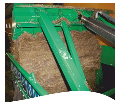
The length of chop can be adjusted. The horizontal chopping knives can cut the bale into up to six slices. Even frozen feed can be cut.
