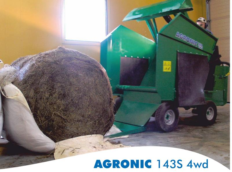
The wrapping and net is cut open before loading. Due to the four-wheel drive, the lift forks slide under the bale effortlessly.
