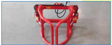
Balehandler specially developped for logistic processing of midibales.
