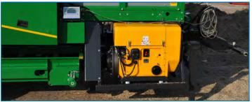
Cost effective operation through a direct connected diesel engine with low fuel consumption. Engine installed as a silent pack on the baler which makes use very simple as well mobile as stationary.
