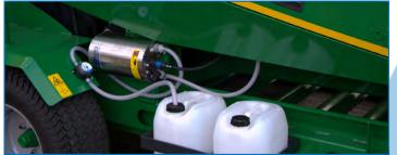
Fully automatic additive system voor adding additives during baling. Pump capacity 10 l/min. Controlled and operated by AGRONIC control unit.
