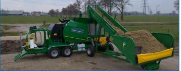
When loading capacity is a requirement, a drop bunker gives a solution. Loading volume is 2,5-3 ton. Direct unloading from wagon into bunker.
