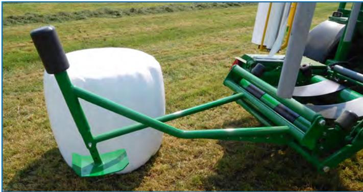
By means of the sidetip the machine automatically unloads the bale on the side. The sides of the wrapped bale have multiple film layers, so damage should be prevented by a hard stubble.
