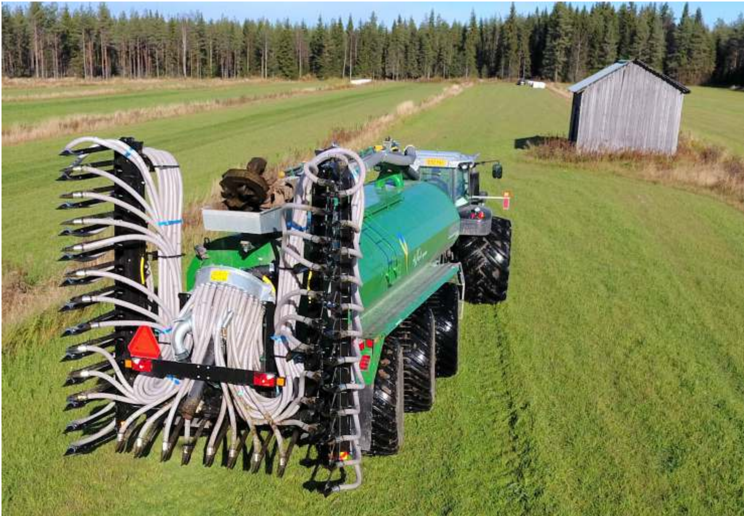
The transport position is compact, the wing turning is automated.
