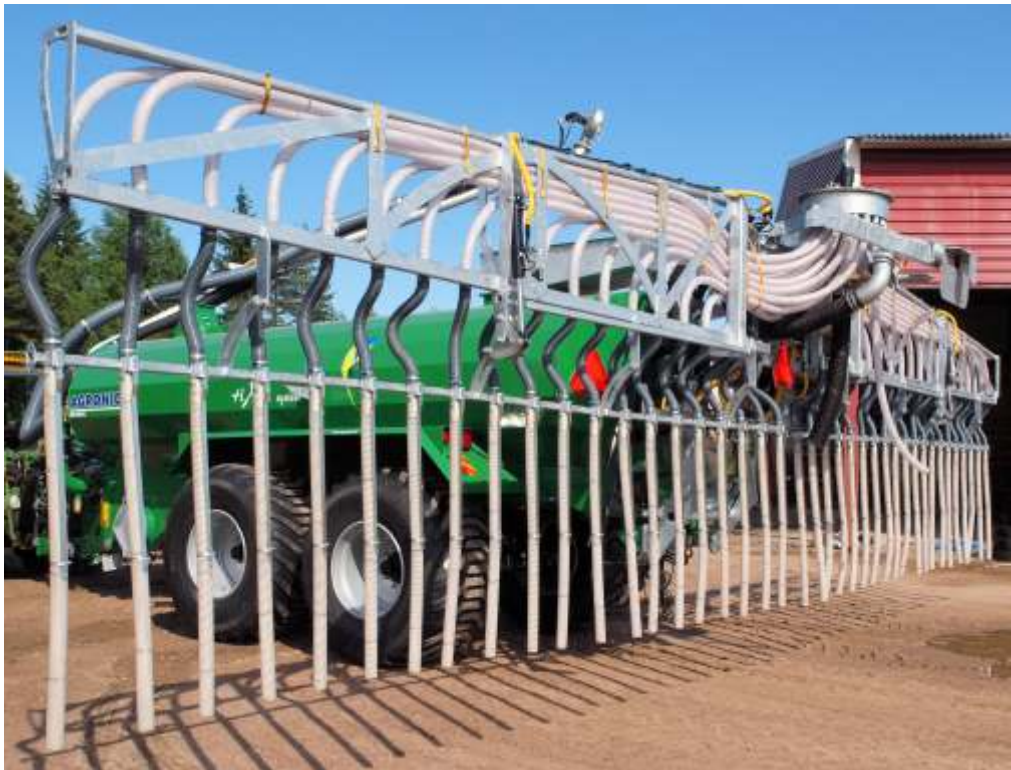
The transport position is compact, the wing turning is automated.
