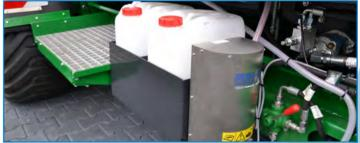
Fully automatic additive system voor adding additives during baling. Pump capacity 10 l/min. Controlled and operated by AGRONIC control unit.
