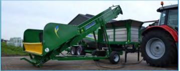
When loading capacity is a requirement. Loading volume is 2,5-3 ton. Conveyor width 1,20 mtr. Direct unloading from wagon into dropbunker.
