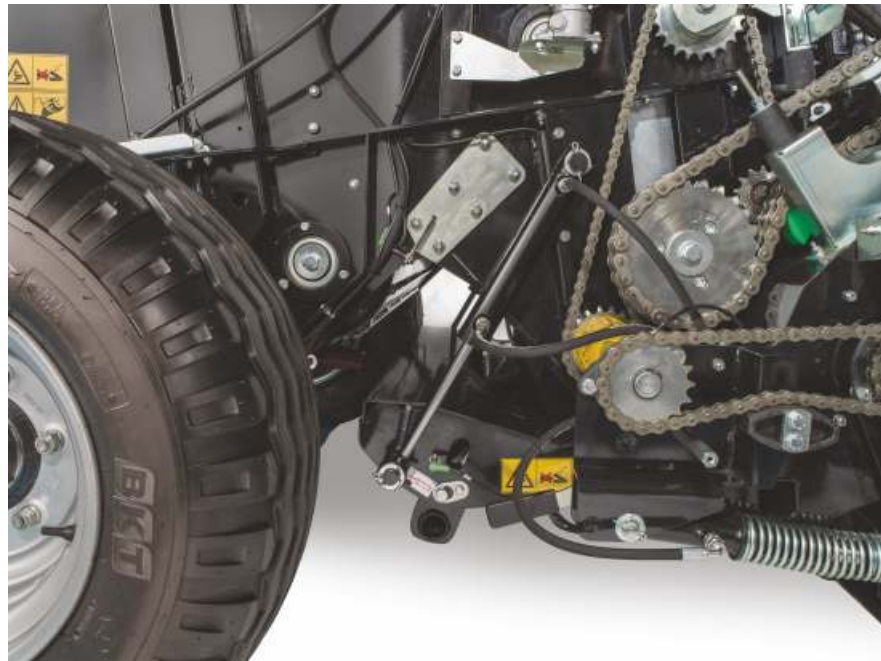
Robust transmission distributes the power to both sides of the baler. On one side to the pick-up, while on the other side to the rollers.
