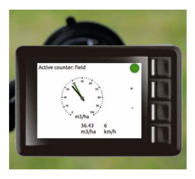
C-Control, flow meter and 3.5" display located in the tractor cab.
