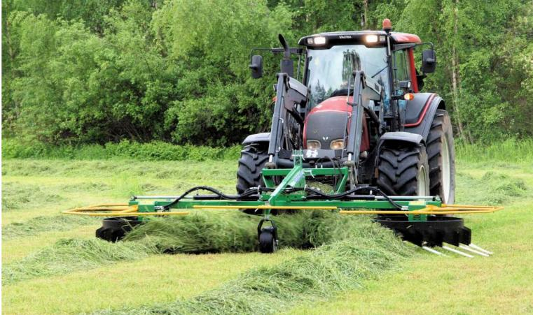
Technicxal DataWr500Wr600Weight (kg)395860Max. Working width (m):5,16,1Transport width (m):3,3, hydraulic telescope2,8, lifting the wings
