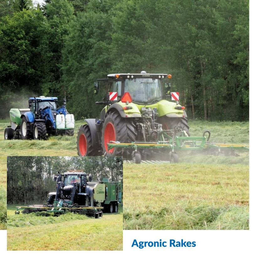
Two models of Agronic windrowers are available. WR500 for front mounting, WR600 for front/rear mounting.
