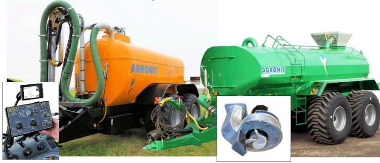
Agronic Fg series, two sizes: 15.5 and 18.5 m3. Due to the shape and construction of the fiberglass tank body, both the center of gravity and the unladen weight are low.
