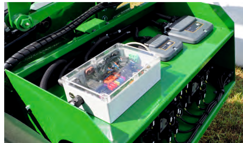
Factory-installed, in-house manufactured, PDH-10 additive application system.
