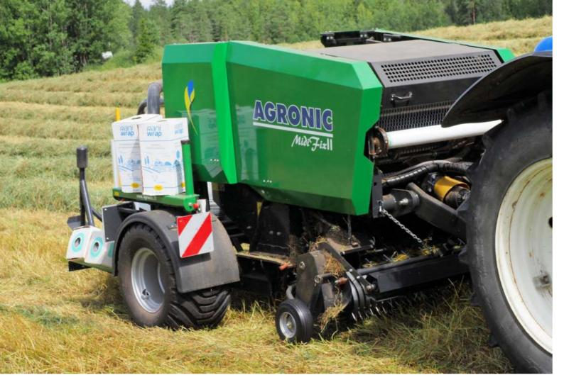
The Agronic MidiFix II bales, transfers, and wraps quickly and reliably. The capacity is up to 70 bales per hour. The operation of the baler is automatic. For possible errors, such as a tear in the plastic wrapping film (or when a film roll is depleted), there are intelligent monitoring systems. The standard rear-facing wide-view camera system improves user comfort and work safety.
