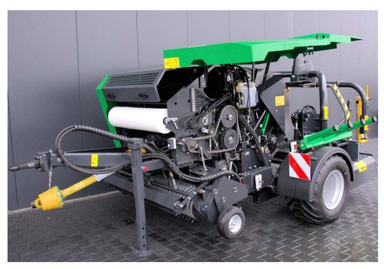
A wide-angle PTO shaft equipped with an overload clutch transmits the power to the bevel gear, which further transfers the power via heavy-duty chains. The chains have automatic central lubrication.
