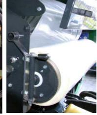
The Agronic MidiFix II ties the bale with a net as standard, a plastic film binding system is available as an optional accessory, and can be used for either net or film binding.
