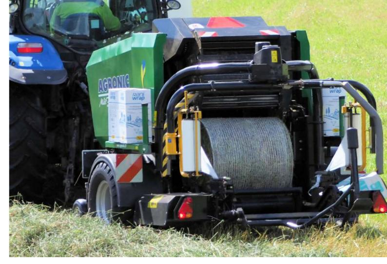
The Agronic MidiFix II can be equipped with an automatic PDH preservative application system, bale weight, moisture measurement system, and comprehensive reporting. This optional equipment also helps to learn the optimal driving speed, as well as the soil moisture levels affecting the crop. The moisture and weight of each bale is shown on the screen after completion, and the information is stored in the memory location.
