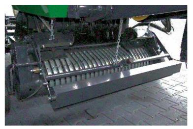
The pick-up has a working width of 1.7 m. There are effective transfer augers on both sides.
