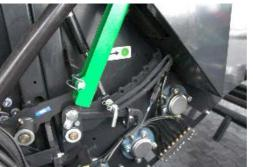
Bale tightness is adjusted by adapting to the angle of the gas cylinders with a 5-position variable mechanical adjustment.
