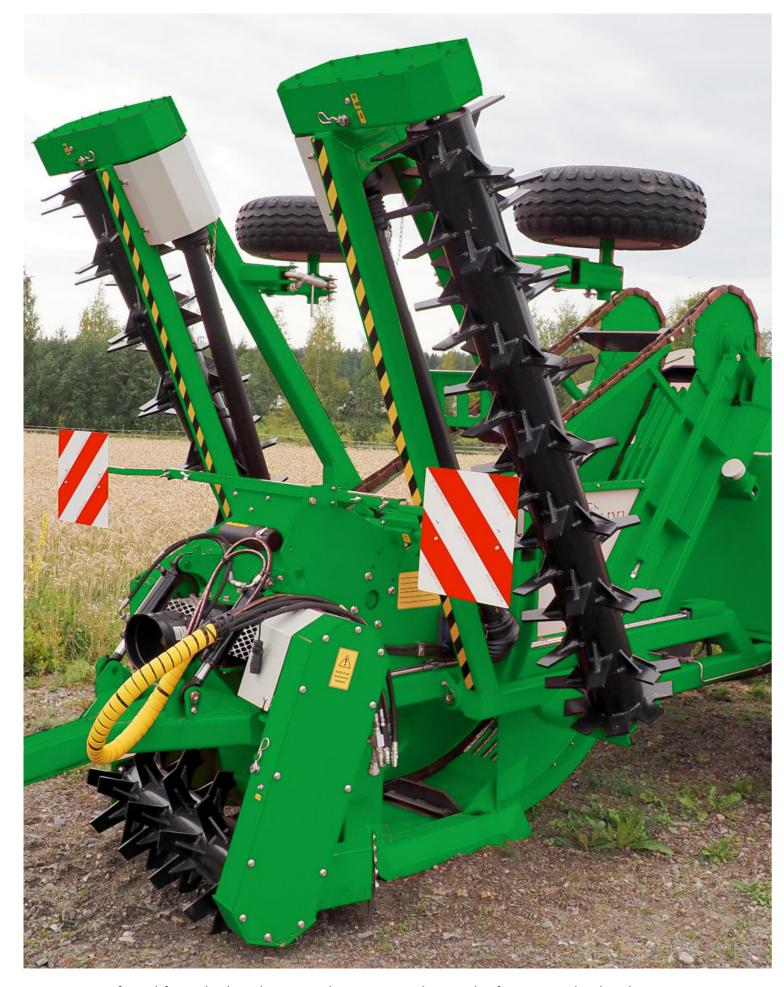
Power is transferred from the bevel gear and main T-gearbox to the front rotor, by the chain transmission and disc clutch.
