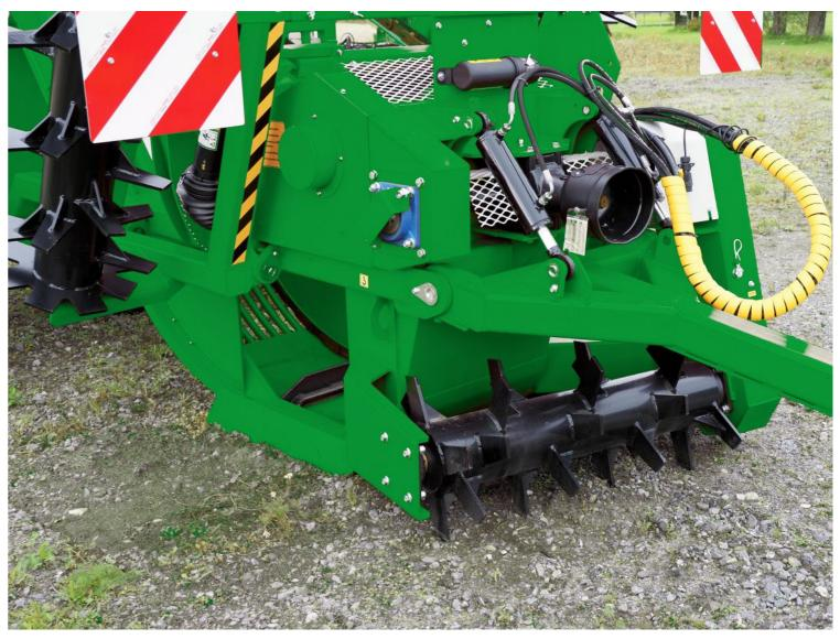
The front rotor processes the soil at a normal working depth at the center of the machine. It does not push the stones into the ground, but the lifts them out. The field surface is also flat at the center of the machine.
