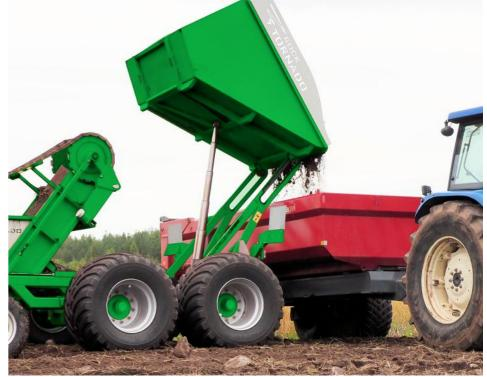
The conveyor moves the stones along the top, dropping them into the hopper. Lifting height of the hopper is 250-cm (8').
