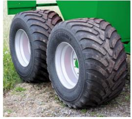
Load-bearing steel belted tires and a strong undercarriage make for good handling in the field and on the road.
